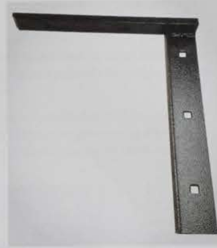
CounterBalance Concealed Brackets from Chemical Concepts are low-profile brackets that provide a clean, floating appearance for the countertop. The brackets are hot rolled, 1/8" steel with a powder-coated finish in black or white, and are available with 9", 12", 18", 24" and 30" support arms. Circle No. 156 on Product Card
