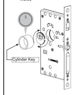
Note: Notches on cylinder must be parallel with the horizontal plane when screwed flush into lock body.
